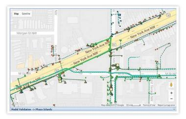
These are sometimes undocumented or lost which can cause significant challenges in safety and in managing the distribution system. NMV testing identifies any loops that are outside of a substation and along all the radial feeders. Any loops detected along the feeder are identified and reported by NMV, which can be used to correct the data in the source system.
